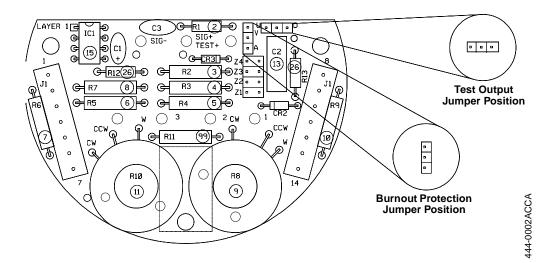
FIGURE 3-2. RTD Transmitter Calibration Diagram.
